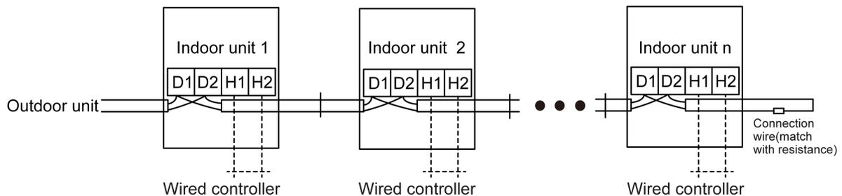
**NOTICE** Indoor unit quantity n is according to the outdoor unit capacity.
