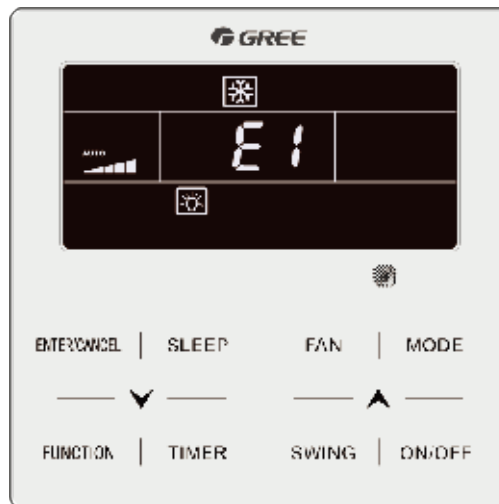
Power-on High-pressure Protection Fault Interface
