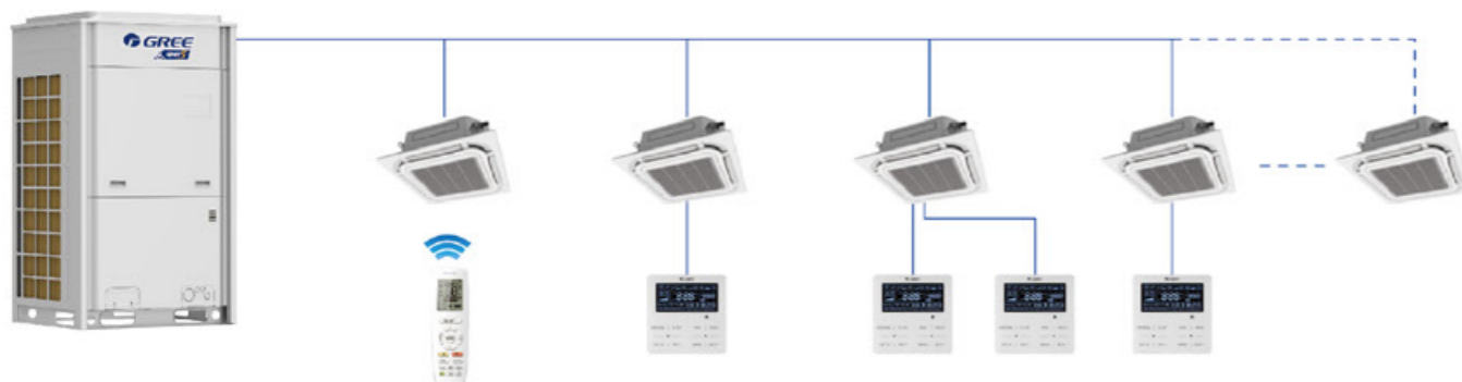
Single control of one unit (Wired controller and remote controller control the unit jointly or separately)
